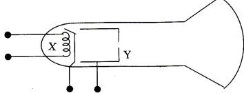
The above diagram shows an electron gun of a hot cathode ray tube,
